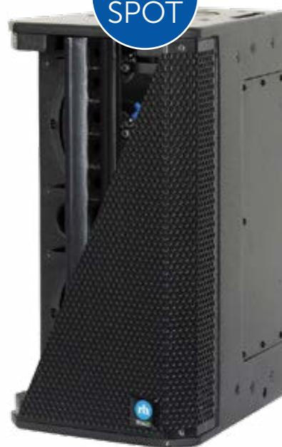
*The Renkus-Heinz ICL-X is fully steerable down to 1500 Hz, and its dual woofer arrangement maintains significant pattern control down to lower frequencies. The ICL-X is a highly versatile loudspeaker and is intended to be used as a high output digitally steerable line array module in array combinations with the ICL-X and ICL-XS up to 12 boxes tall.*
